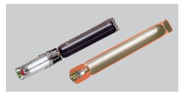
The ASH-2 inflator (to the right) uses a completely new principle for airbag inflators: Dissociation.
