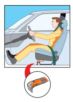
the impact by gradually ripping apart. The seat then pivots rearwards in a controlled manner instead of violently pushing the occupant's shoulders and lower neck forward.
