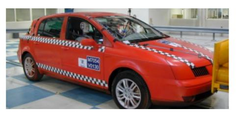
Autoliv France has expanded its technical center by adding a new track for full-scale test where complete vehicles, weighing up to four tons, can be crash tested at speeds up to 80 km/h or vehicles weighing two tons can be tested at 120 km/h. The tests are not only frontal, but also rear, side and car-to-car. Since the opening in May 2000, more than 150 fullscale tests have been performed in the new crash lab.
