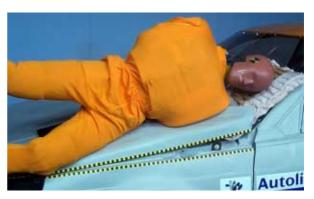
Autoliv's Active Hood (left) and Pedestrian Protection Airbag (right) improve the safety for pedestrians by reducing the risk of a person hitting the hard car structure, the base of the windshield or the windshield pillars
