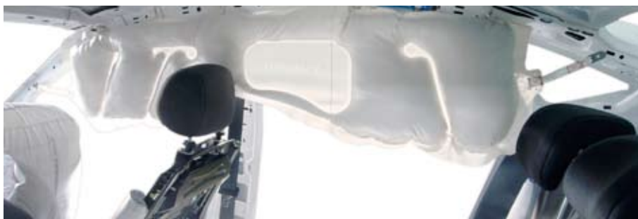
Curtain airbags make up the fastest growing product segment on the market. They can reduce the risk of fatal head injuries by as much as 50%.
