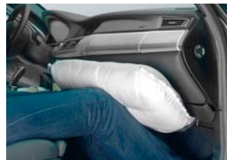
Knee airbags can help prevent long-term disabling injuries which is very important for the increasing number of occupants now surviving crashes.
