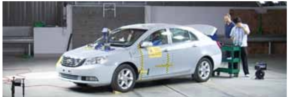
A vehicle under preparation for full-scale crash test in Autoliv's new technical center in Shanghai, China.
