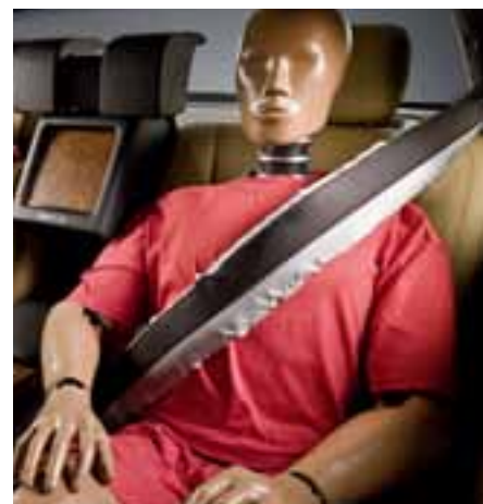
The Belt Bag, developed together with Mercedes-Benz for their Experimental Safety Vehicle, is a combination of a seat belt and an airbag. This product will practically double its width within fractions of a second during an accident, thereby distributing the load on the occupant over a wider area, to reduce the risk of injury. This is particularly beneficial for older passengers, whose ribcage may no longer be so flexible. (Image credit: Daimler).
