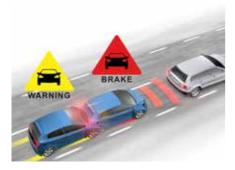
Autonomous Emergency Braking (Radar or Vision) Continuously monitors the area in front of the vehicle to detect slow moving vehicles and other objects.
