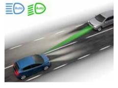
High/Low Beam Assist (Vision) The system identifies on-coming vehicles and determines when the head lights need to be dipped in order not to blind the on-coming driver.
