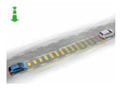
Adaptive Cruise Control (Radar) Automatically adjusts the vehicle speed to maintain a safe distance from vehicles ahead.
