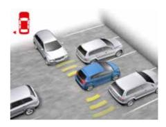
Cross-Traffic Assist (Radar) Helps detect cross traffic when reversing out of a parking space.
