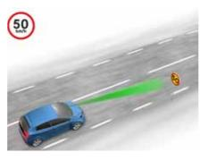
Traffic Sign Recognition (Vision) The system keeps the driver informed of the speed limit and other traffic signs on the road.
