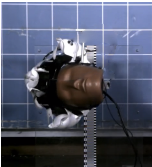
The drop Test. The height was either 1.5 or 1.8 m in these prestudy tests.
