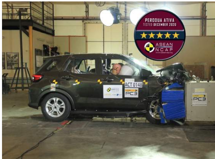
Figure 2.4.5. ASEAN NCAP crash test at PC3 Lab
